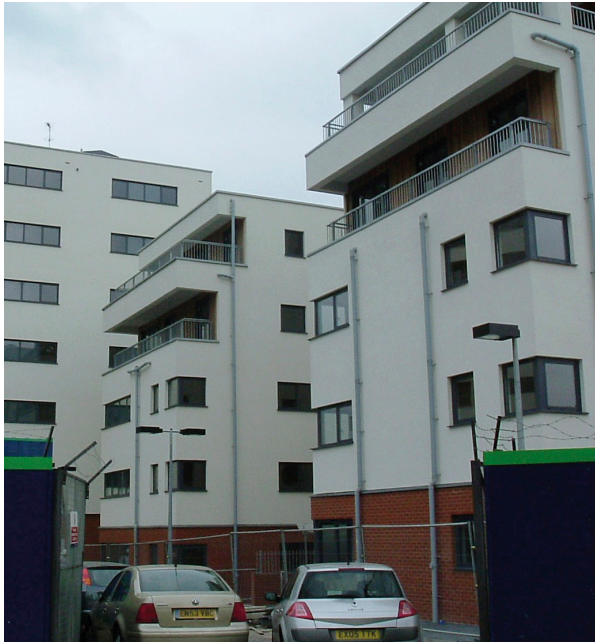
Figure 8: A white finish to external walls, as in this North London development (architects Sheppard Robson), can increase reflected light. However, windows will tend to reduce the overall effective reflectance.
