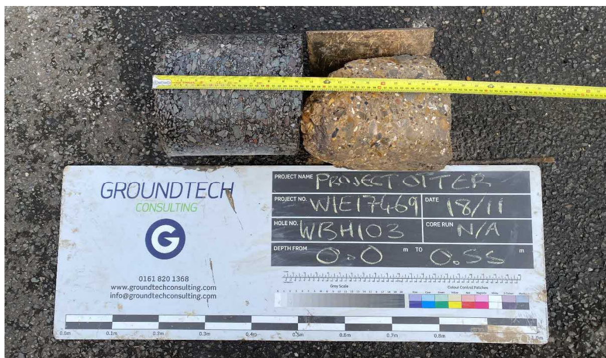
Photograph 7 – WBH103 tarmac and concrete cores.
