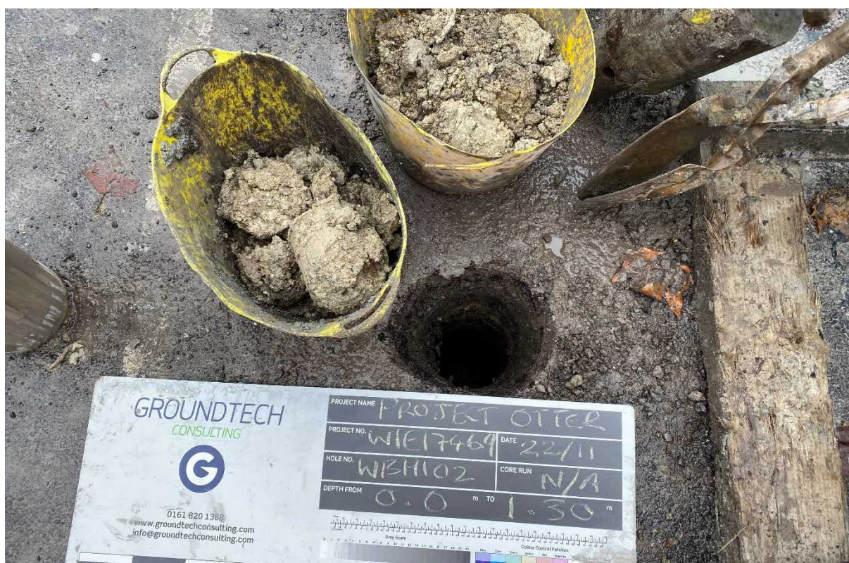
Photograph 6 – WBH102 Inspection pit
